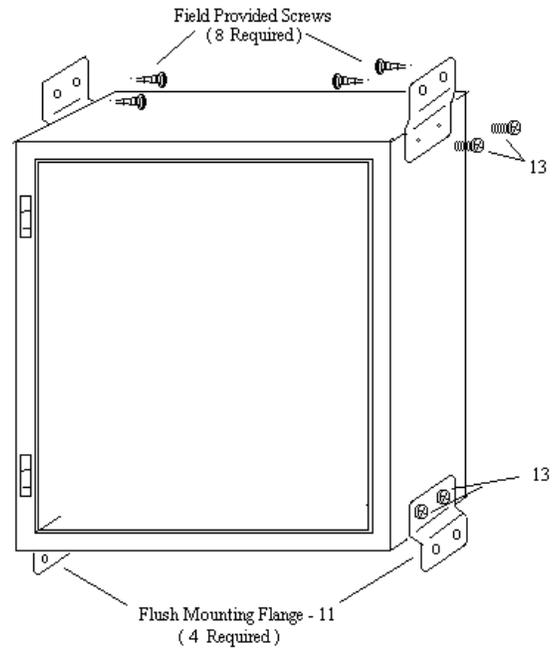
**Figure 2** For best Flush Mounting results, recess face of enclosure's lip 1/4" behind wall finish
