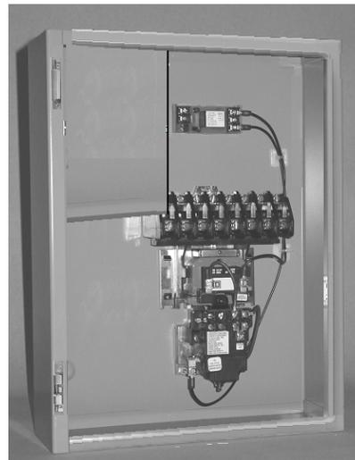
The *ISIMET* Laboratory Service Panel operates as a single output controller incorporating either a solenoid valve assembly or electrical contacts along with the digital switching mechanism within a single enclosure. An internal junction box houses the 120-vac line voltage along with transformer and circuit board.
