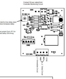
If the unit is provided with a Time Delay "ON" circuit board, make wiring connections as shown in the drawing above. Units W/ Lamp & Horn: (typical) WHT – COM BLK – Horn (N/O terminal) Blue – Lamp (Immediate terminal)
