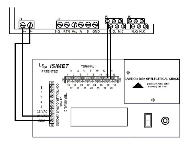
CAUTION: Do NOT run dry contact wiring from J1 & J5 in conduit with any voltage carrying wiring. Each voltage carrying wiring should be run in its own conduit.
